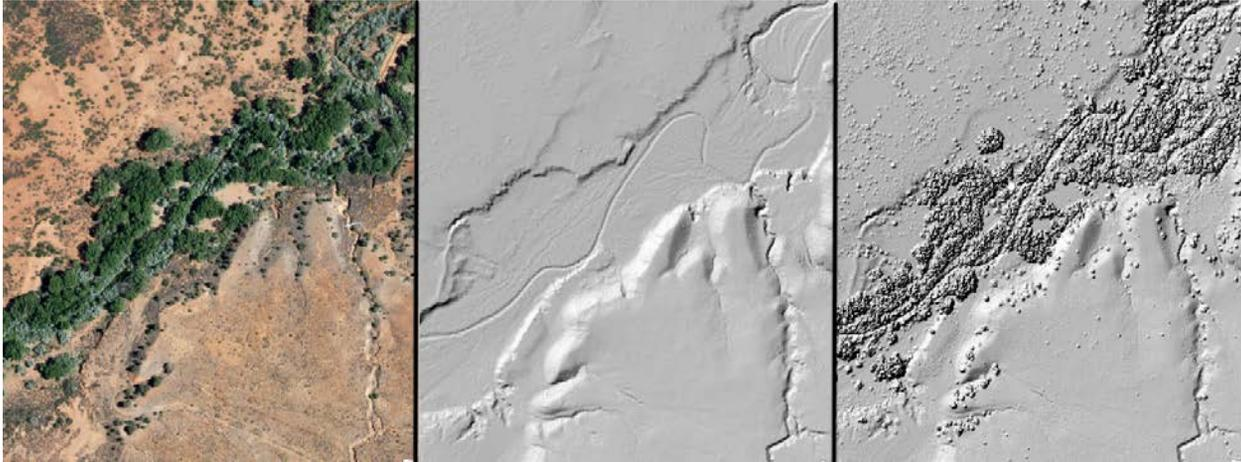
*2020 NAIP**LiDAR Derived Digital Terrain Model**LiDAR Derived Digital Surface Model*
