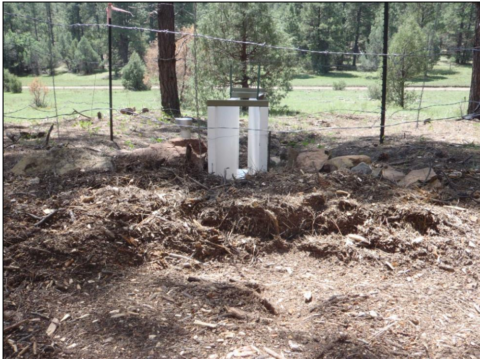
Figure 2.34. The flume on the treated Chilili site clogged with pine needles and wood chips following a flow event that occurred on August 20, 2011.
