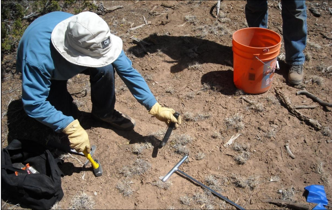
Figure 2.27. Soil cores were taken using an impact corer, shown above, for chemical analysis.
