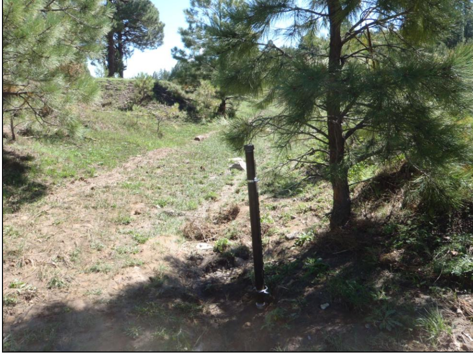
Figure 4.4. The new Chilili piezometer that was installed in the fall of 2011 to replace the storm damaged gauge.
