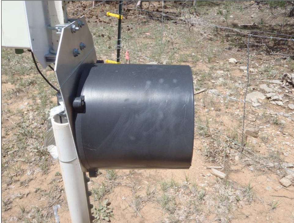
Figure 2.12. Damage to the tipping bucket rain gauge caused by a black bear on Chilili Control Plot.
