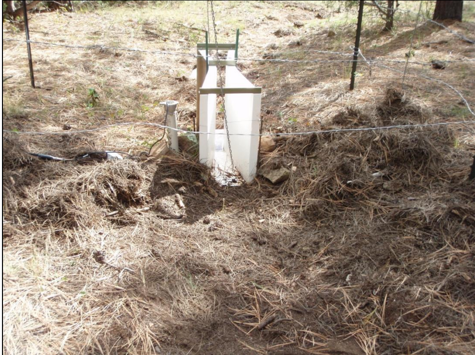
Figure 2.32. Parshall flume located at the thinned Chilili site.
