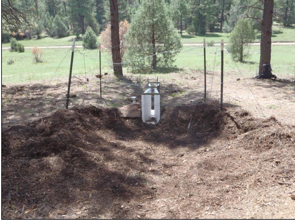
Figure 2.35. The flume on the treated Chilili site after the pine needles and wood chips were removed from the throat, following a flow event on August 20, 2011.
