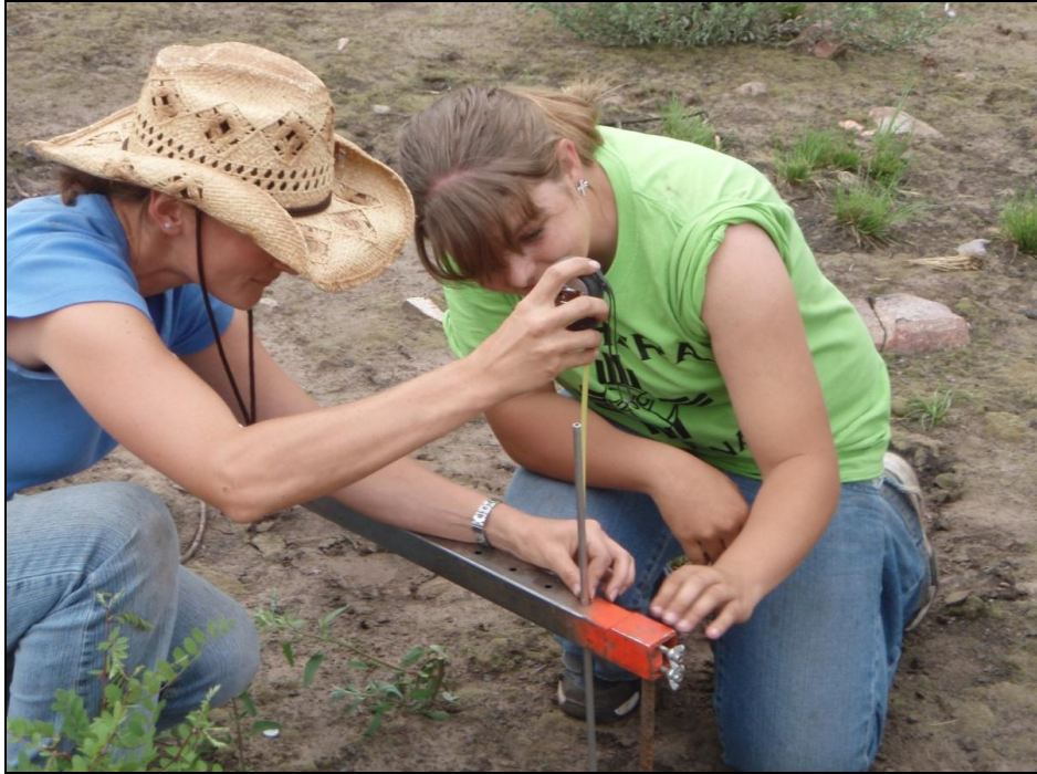
Figure 2.24. Measurement of soil surface topography using a soil movement bridge helps understand the yearly variability associated with soil topography.
