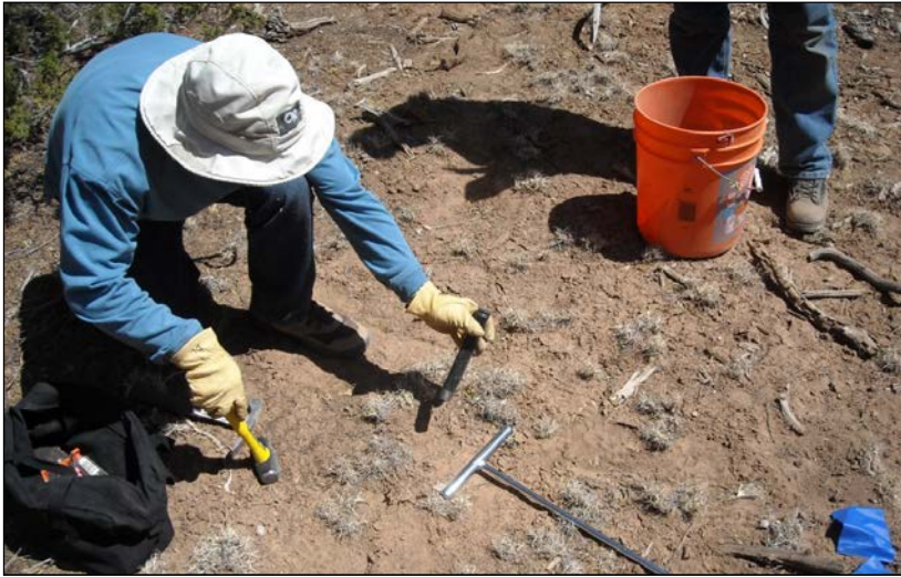
Figure 2.39. Soil cores were taken using an impact corer, shown above, for chemical analysis.
