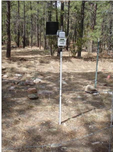
Figure 2.7. WatchDog mini weather station at the Wester ponderosa pine site.
