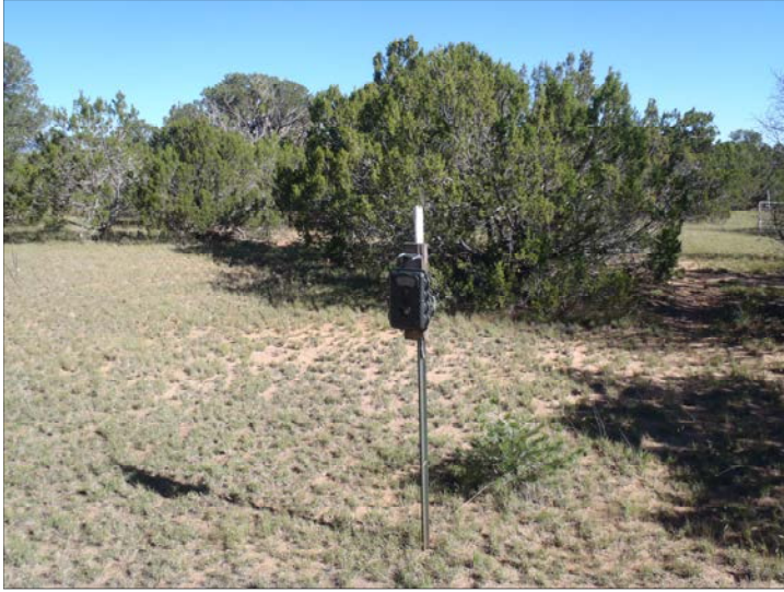
Figure 2.83. Automatic wildlife camera (Truth Cam, model 63010).
