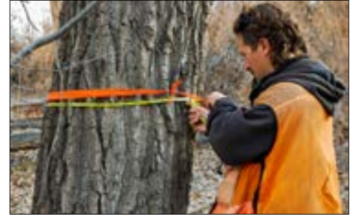
Alex Makowicki takes the measurement of a tree trunk diameter as part of calculating the woody mass in a plot. Photo by Jake Robinson/NMHU Media Arts
