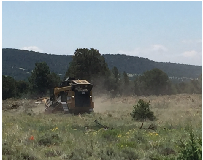
A masticator at work on a CFRP project on Rowe Mesa.
