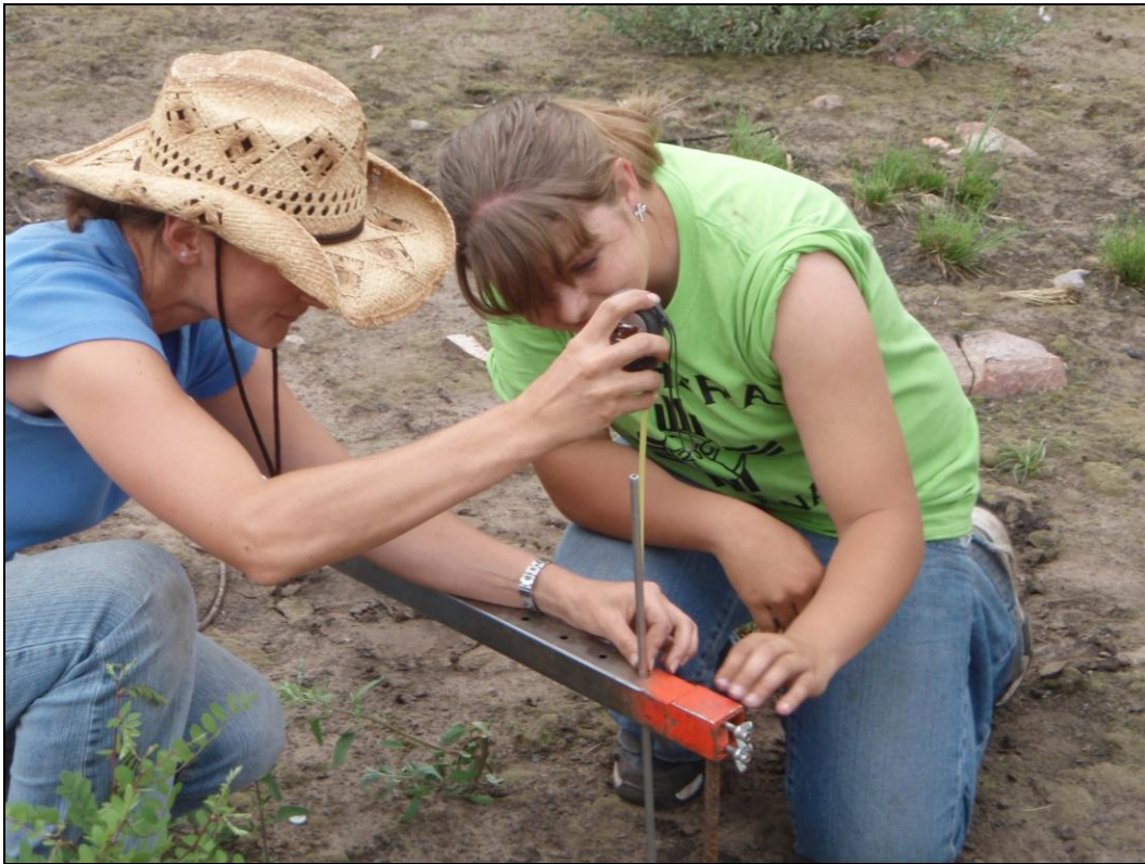
Figure 2.15. Measurement of soil surface topography using a soil movement bridge helps understand the yearly variability associated with soil topography.
