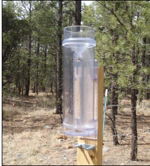
Figure 2.2. Graduated rain gauges are used for backup in the case of failure from one of the WatchDog weather stations.
