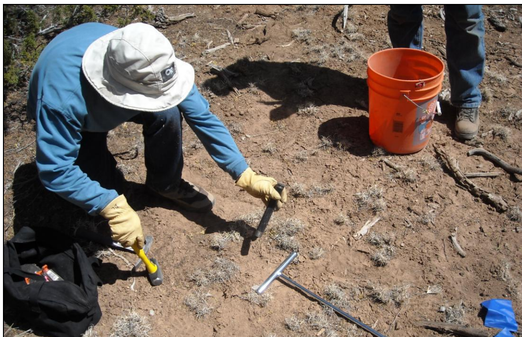
Figure 2.18. Soil cores were taken using an impact corer, shown above, for chemical analysis.
