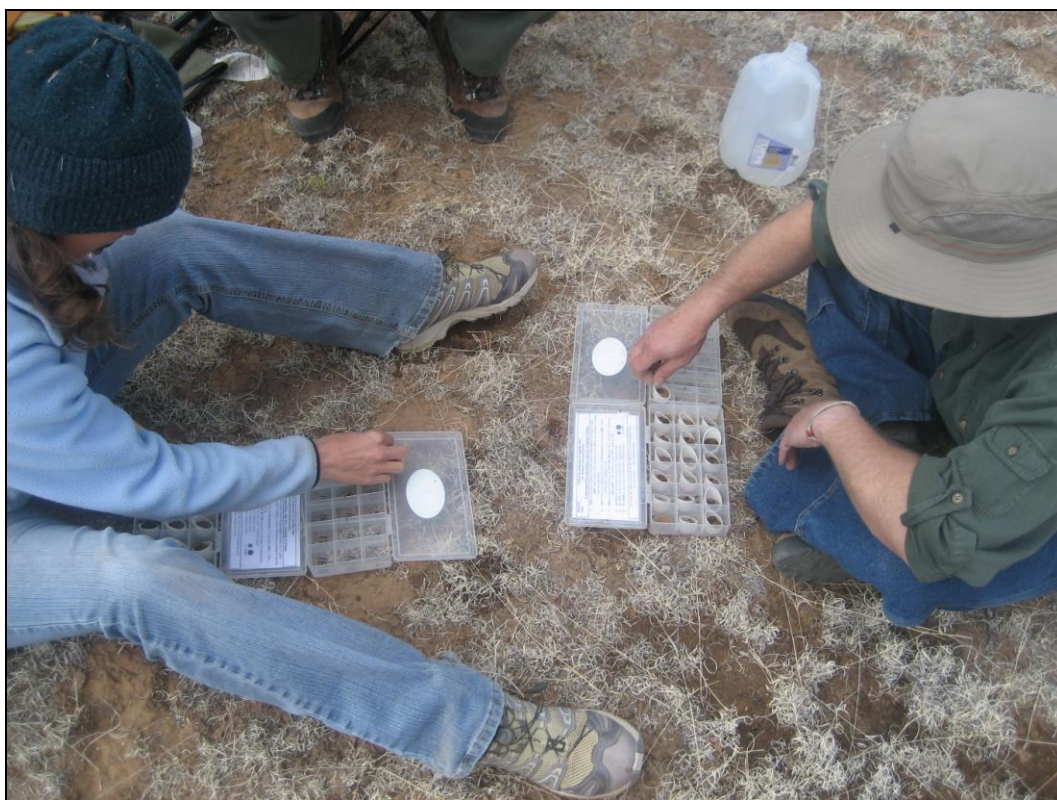
Figure 2.12. Soil stability test in use on the study sites.
