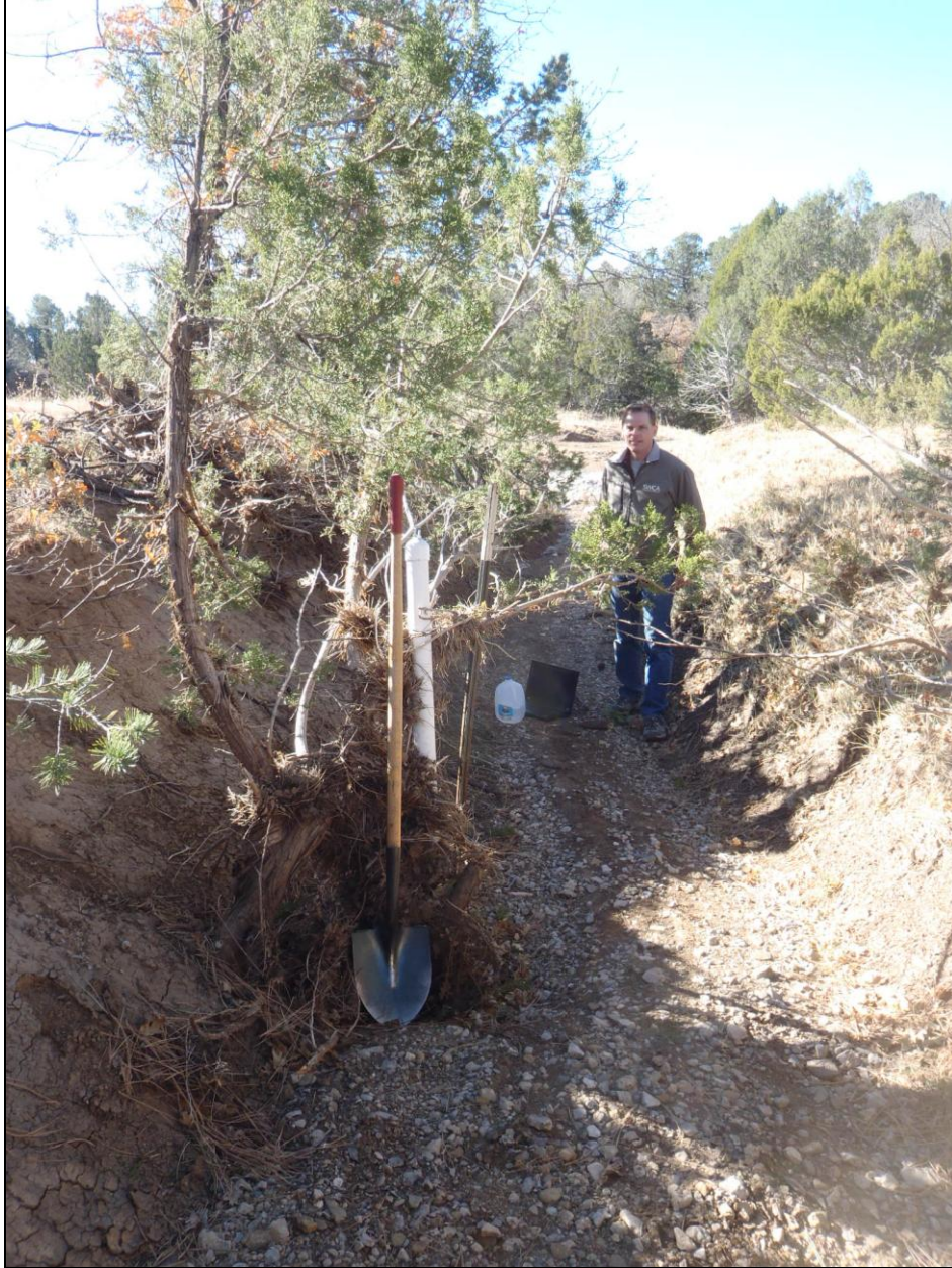
Figure 4.3. The Vigil piezometer in the fall of 2010 after a storm event lowered the stream bed level to below the piezometer. The shovel shows the location of the high water line determined by the accumulation of debris in the vegetation.
