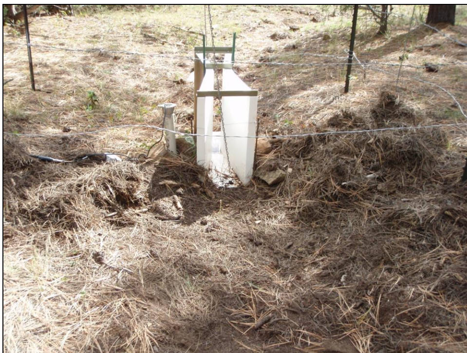
Figure 2.23. Parshall flume located at Chilili site plot 1.
