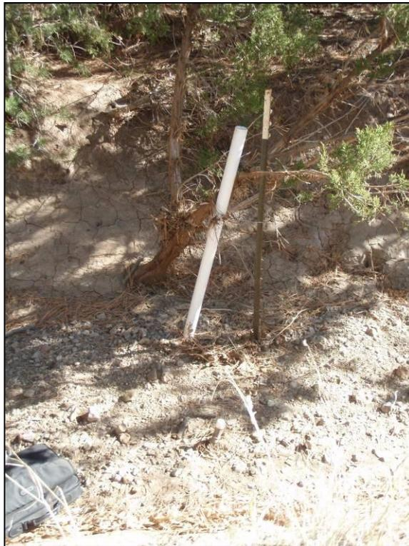
**Figure 4.5.** Large amounts of deposition and debris accumulation at the Vigil piezometer after a storm event in 2008.
