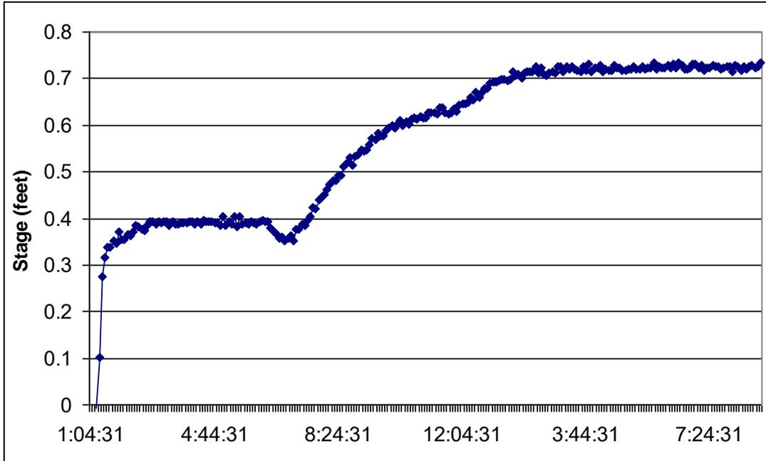
**Figure 4.2.** Hydrograph from the Candelaria piezometer on September 17, 2009, showing a peak stage of nearly 1 foot. However, notice there is no decline to the peak, which is likely caused by the sediment accumulation seen at the site.
