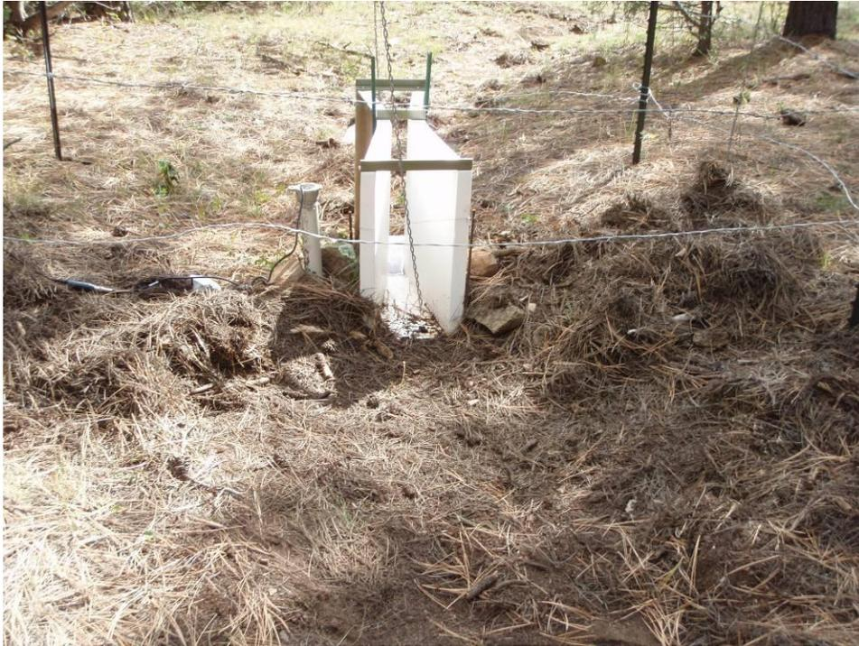
**Figure 2.29. Parshall flume located at Chilili site plot 1.**
