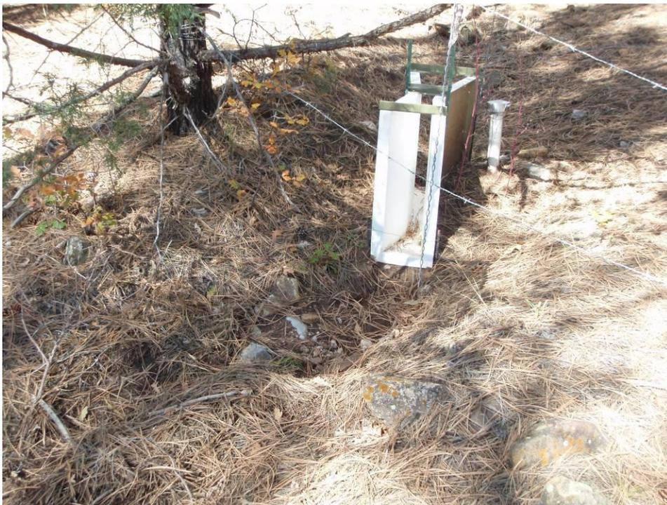
**Figure 2.30. Parshall flume located at Chilili site plot 2.**
