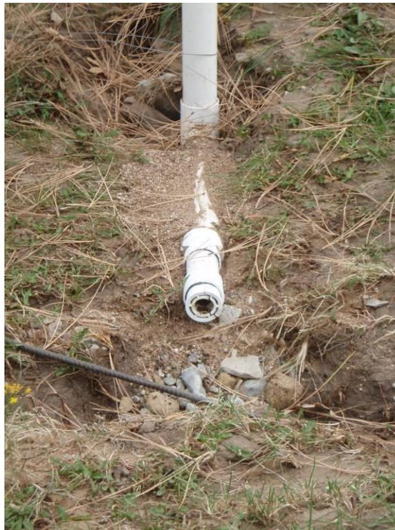
**Figure 4.7.** Damage to the Chilili piezometer in 2009. Even though the end cap was removed, this piezometer was still able to record flow.
