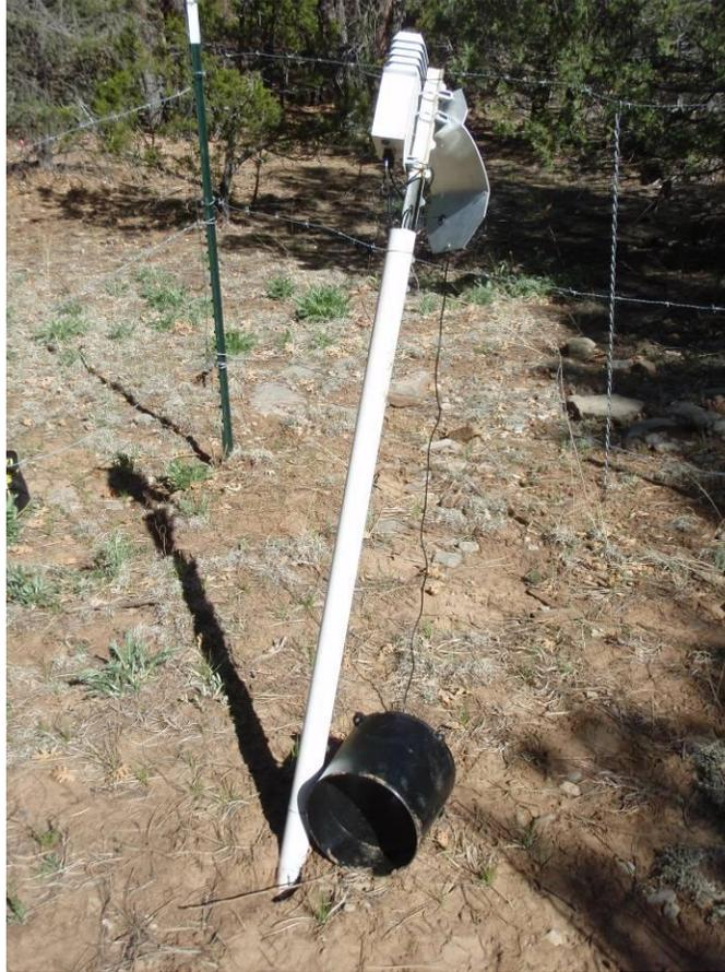
**Figure 2.5.** Photo taken in April 2009 showing initial bear damage caused to the WatchDog station.
