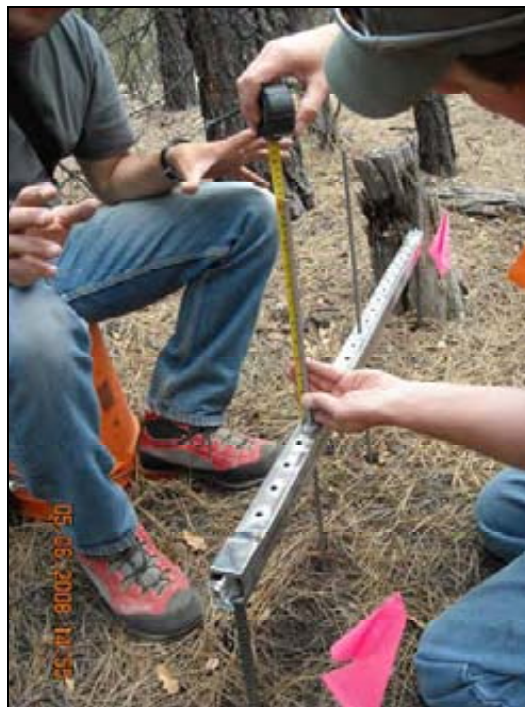
Figure 75. Soil erosion bridge measurements.
