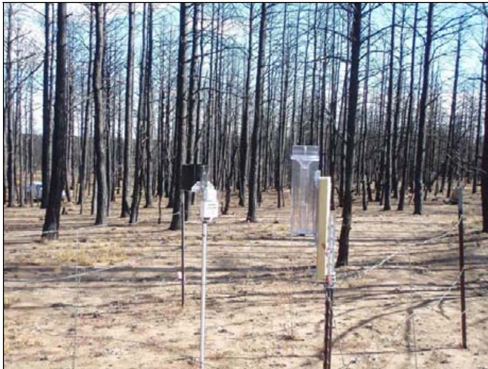
Figure 28. WatchDog Mini Weather Station and a graduated cylinder as a backup to collect precipitation data. These stations have been installed at each forest thinning plot and near fire monitoring plots.
