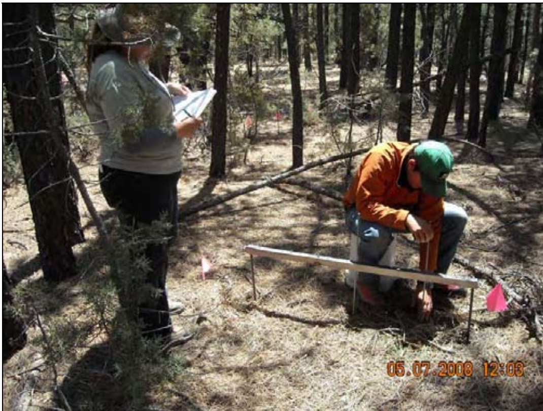
Figure 16. Soil erosion bridge measurements being taken.
