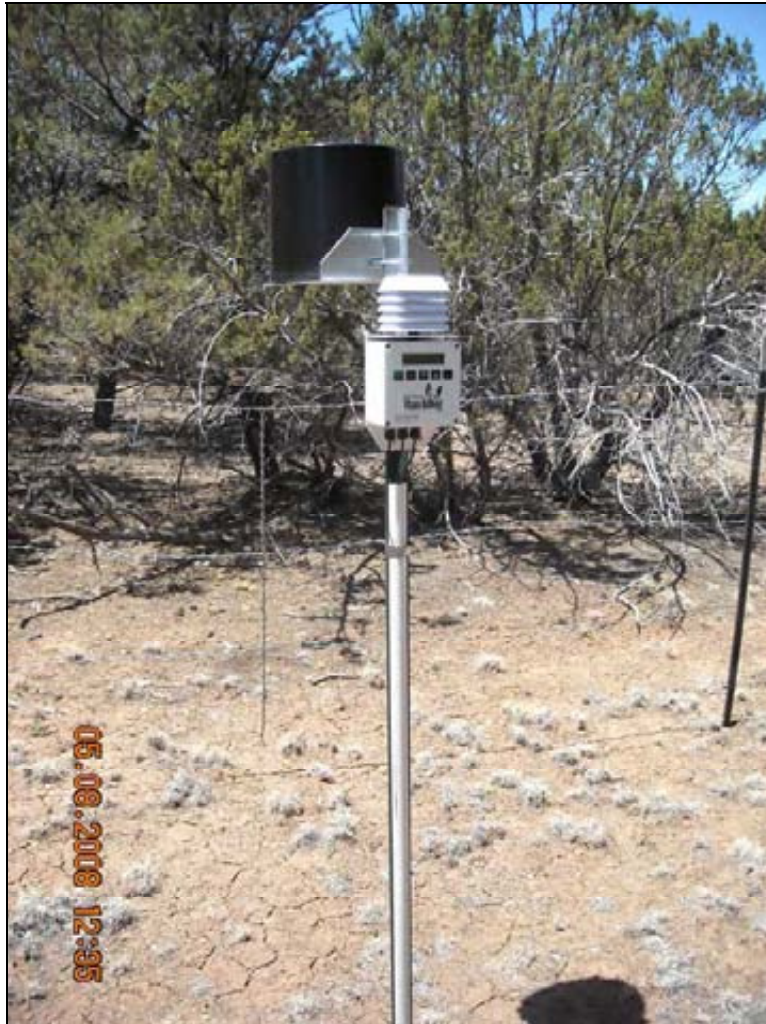
Figure 4. WatchDog automated Mini Weather Station.
