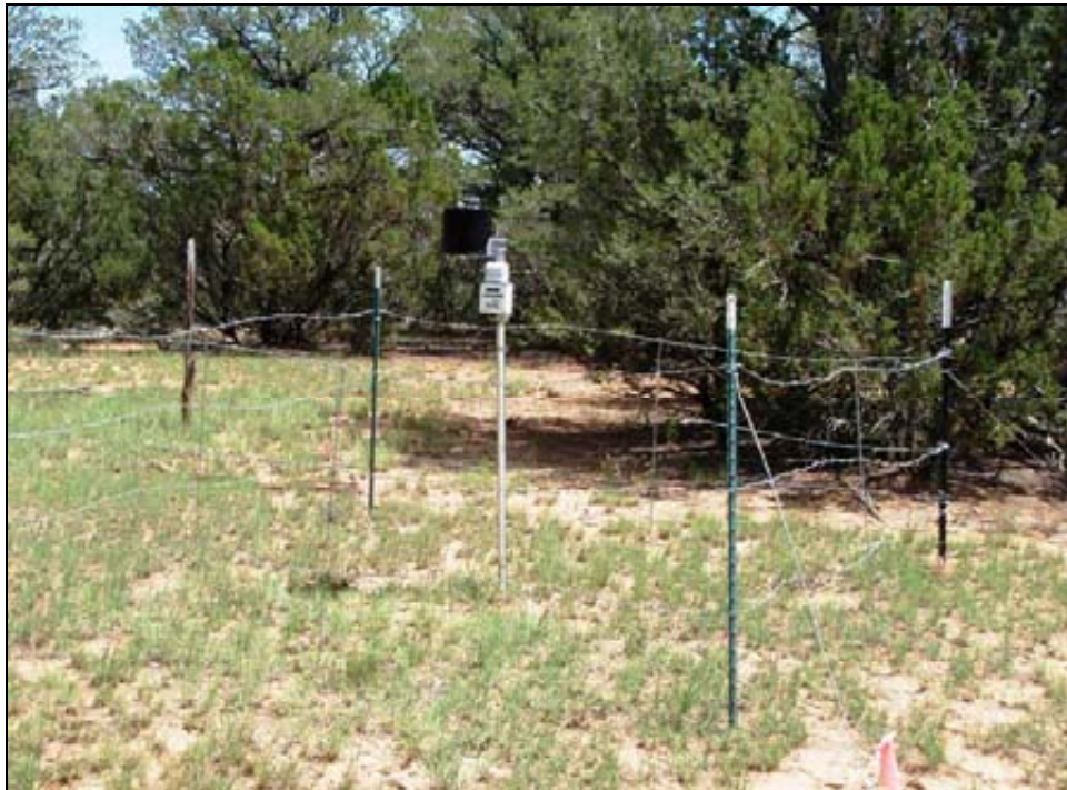
Figure 91. Vigil WatchDog Mini Weather Station.
