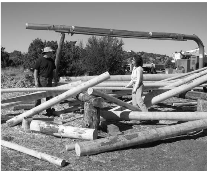
Figure 2. CFRP grantee Gordon West and former Gila National Forest CFRP coordinator Kim Hunter discuss the use of a log peeler in Silver City, New Mexico. These ponderosa pine logs are peeled and sold as vigas (ceiling poles) that are popular in southwestern construction.
