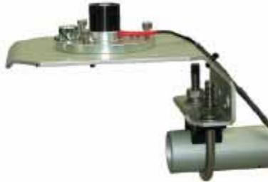
The pyranometer sensor surface should be cleaned with a blast of compressed air monthly and the leveling checked regularly. The pyranometer also requires a biannual factory recalibration.
