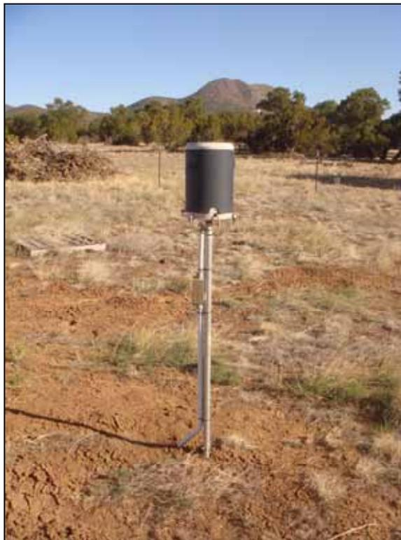
**Figure B.5. Rain bucket with insulation.**
