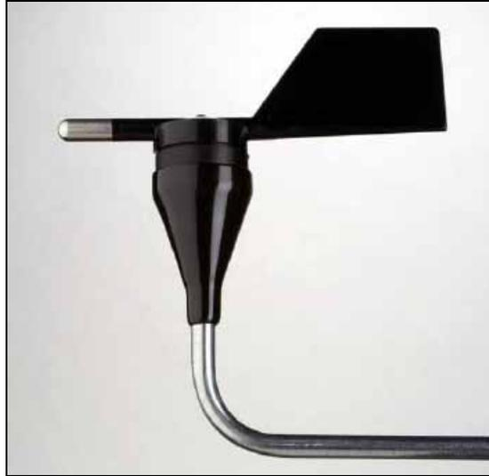
The wind direction vane operates using a potentiometer (essentially a dial) which that transmits a specific electrical potential for any direction within the 360 degree range. For example, if the wind is blowing from the north the potentiometer should transmit 0 Volts which translates into 0 Degrees (N), but if the wind shifts to the east the potentiometer transmits approximately 3.75 volts which translates to 90 Degrees (E).
