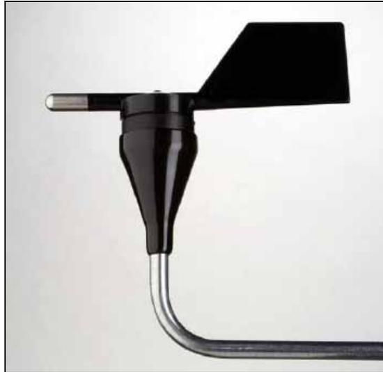
The wind direction vane operates using a potentiometer (essentially a dial) that transmits a specific electrical potential for any direction within the 360 degree range. For example, if the wind is blowing from the north the potentiometer should transmit 0 volts, which translates into 0 degrees (N), but if the wind shifts to the east the potentiometer transmits approximately 3.75 volts which translates to 90 degrees (E).
