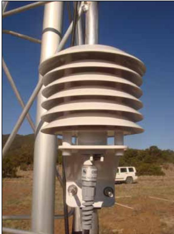
**Figure B.9. Air temperature and relative humidity sensor (with radiation shield).**
