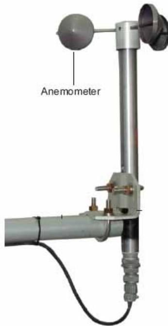
During each revolution of the cups, a switch is opened and closed twice. Wind speed is measured by converting the frequency of switch closures to meters per second or miles per hour (mph). The anemometer can measure winds speed of up to 100 mph with an accuracy of 0.25 mph, but has a starting threshold of 1 mph; it measures from 1 to 100 mph in quarter mph increments or 0 mph (no wind).
