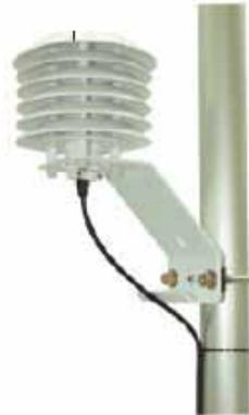
The temperature/relative humidity sensor has a filter that covers the sensor element which requires monthly cleaning and inspection. The filter is replaced periodically dependent on its condition. The sensor element itself must be replaced annually; both of these procedures are outlined in the SMWS Maintenance Manual.
