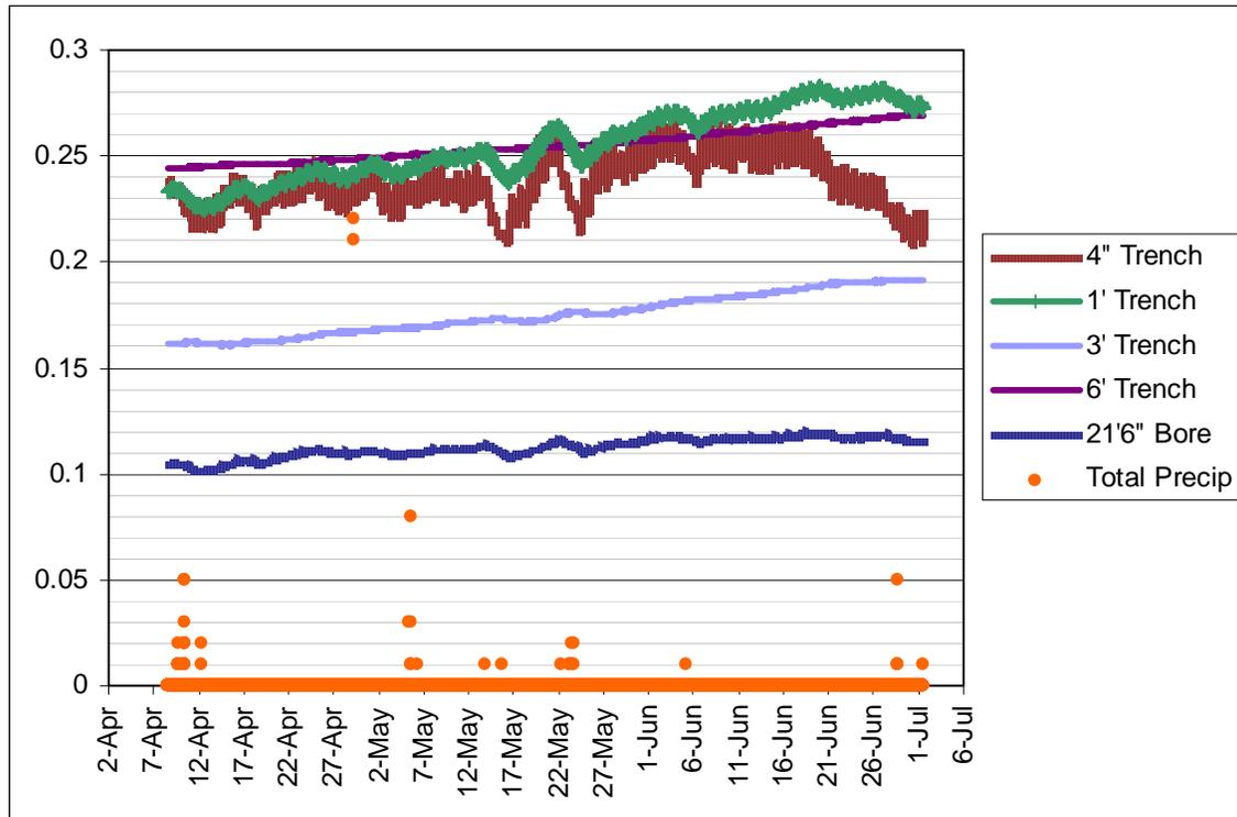
**Figure 34. Tree site soil moisture levels and precipitation, April–July 2008.**
