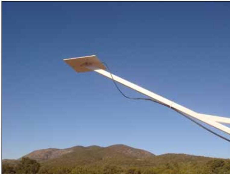
**Figure B.10. Pyranometer with arm.**
