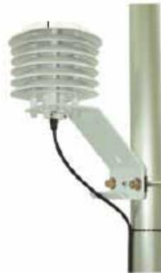
The temperature/relative humidity sensor has a filter that covers the sensor element which requires monthly cleaning and inspection. The filter is replaced periodically dependant on its condition. The sensor element itself must be replaced annually; both of these procedures are outlined in the SMWS Maintenance Manual.
