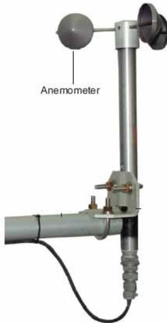
During each revolution of the cups, a switch is opened and closed twice. Wind speed is measured by converting the frequency of switch closures to meters per second or miles per hour (mph). The anemometer can measure winds speed of up to 100 miles per hourmph with an accuracy of 0.25 mph, but has a starting threshold of 1 mph; it measures from 1 to 100 mph in quarter mph increments or 0 mph (no wind).
