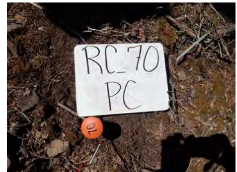
Figure 16. Example of capped rebar marker.
