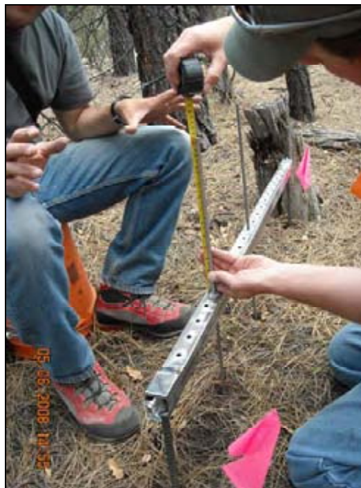
Figure 75. Soil erosion bridge measurements.
